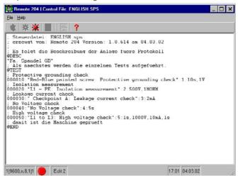
The above sample is used as a model for the creation of new control files. It can be modified and expanded as desired.
